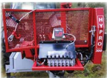
*The machines control table is placed in a comfortable working height and has easily maneuverable levers, where it also is possible to adjust the speed in both directions individually on all functions. The measuring system is optimal placed for a comfortable use.*
