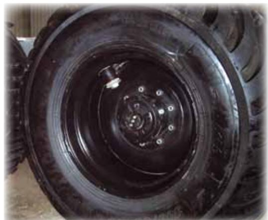
*Hydraulic motor drive via planetary gear generates very strong work force. With the drive activated, the hydraulic motor has automatic free rolling up to 40 km/h with the LS-system. The drive device is placed in the rear wheel pair.*
