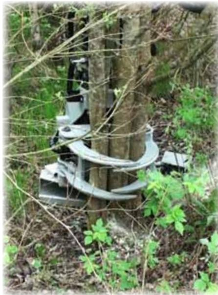
The **HYPRO FG45** felling grapple is ideal for use in the handling of both standing and felled trees. The felling grapple can be mounted on just about any crane with a rotator.
